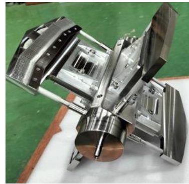
Prototype of the revolver type collimator (atmospheric specifications)
