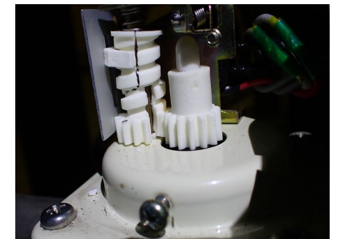
Damaged flow-switch part (POM)
