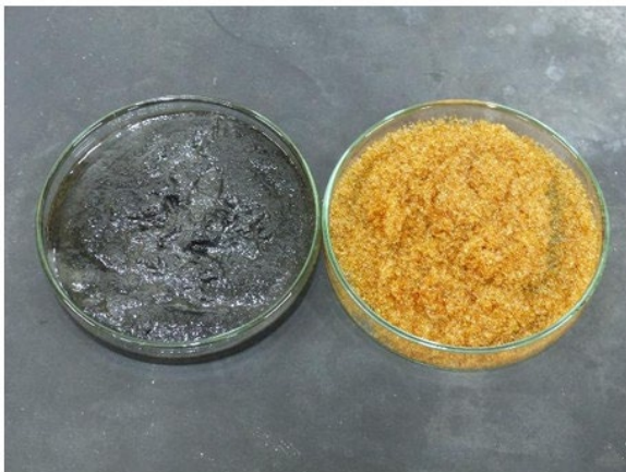
Demineralizer resin samples, 2026. (Left) Used resin, (Right) New resin.
