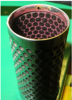
(Left) Needle valve, (Right) Strainer clogged with copper oxide.
