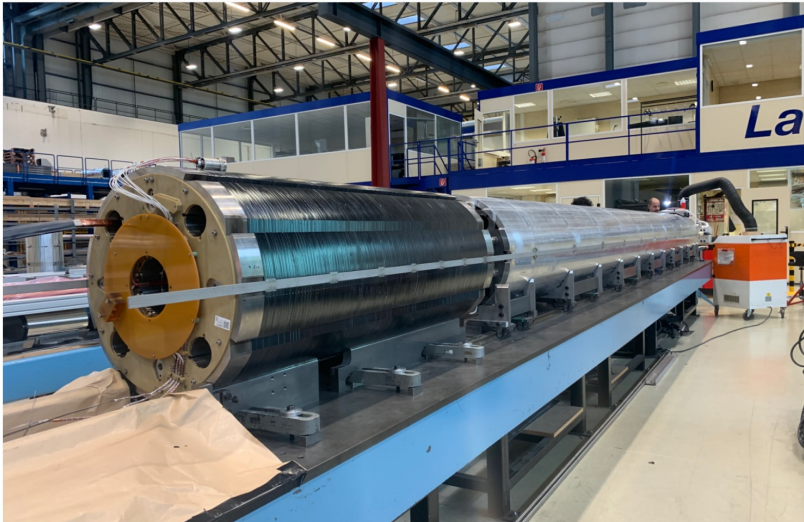
The MQXF BP3 magnet after the test, during assembly with the nested dipole orbit corrector. (Image: CERN)
