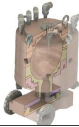
New pulse compressor Spherical-Cavity Pulse Compressor (SCPC)
