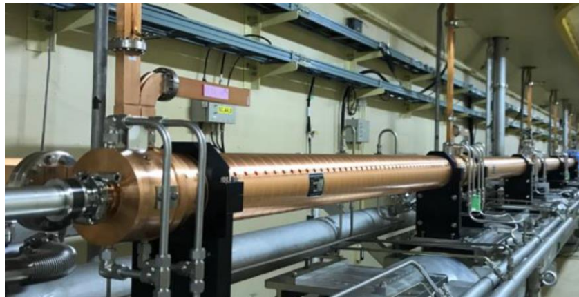
New S-band 2-m-long TW acc. structure
